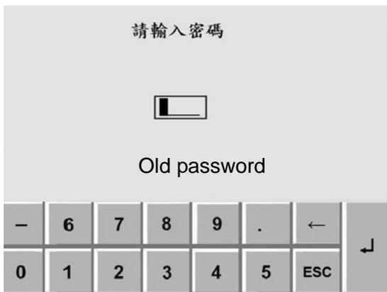
Enters “the password setup” in front of the picture, the controller can request please first to input the old password first, after waits the input to finish presses the enter key then enters “the password setup” the picture again.
