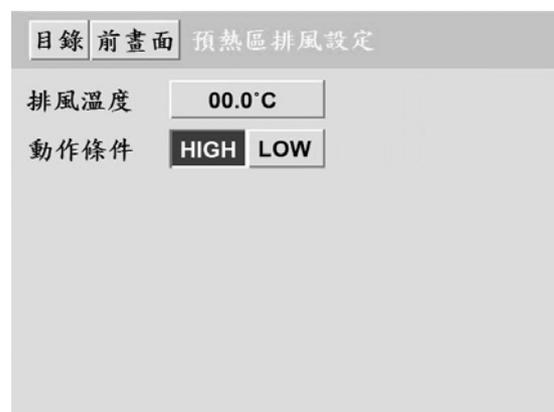
**Control requirement:** According to high temperature temperature SV and row of wind temperature SV the corresponding relationships, decided when [EXHAUST] does contact outputs. When high-temperature test execution, take high-temperature test temperature SV as the determination object; When preheating experimental execution, take preheating temperature SV as the determination object.
